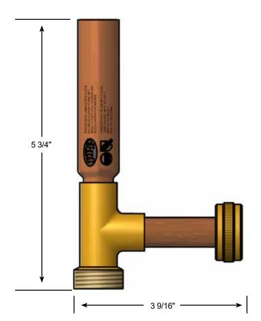
**INSTALLATION**: May be installed in new or existing plumbing systems with a standard pipe tee.
