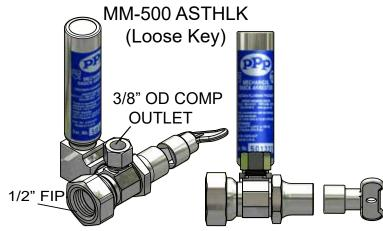
This innovative arrestor series combines an angle stop required for many plumbing fixture applications with a built in water hammer arrestor. The unit is designed to control the damaging effects of pressure spikes caused by quick closing valves within a system. The Loose Key feature replaces the exposed handle provided with other angle stops and provides a degree of vandal resistance in public installations.
