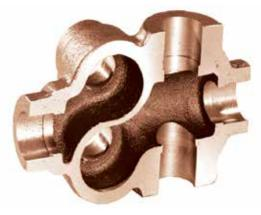
CUT AWAY OF BAC-2-BAC® SHOWING INTERIOR PASSAGEWAYS THAT DISTRIBUTE HOT AND COLD WATER WHERE NEEDED. **BAC-2-BAC® MANIFOLD** distributes hot and cold water to fixtures mounted back to back on partition.
