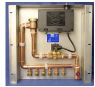
The Electronic Priming Assembly pictured is available in a single configuration but is capable of priming from thirteen to twenty separate floor drain traps from a single control unit. The manifold is available in either 1/2" or 5/8" compression and 1/2" PEX fittings. This model serves 13 to 20 drains.
