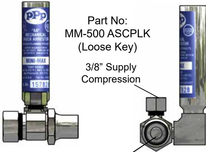
This innovative arrestor series combines an angle stop required for many plumbing fixture applications with a built in water hammer arrestor. The unit is designed to control the damaging effects of pressure spikes caused by quick closing valves within a system. The Loose Key feature replaces the exposed handle provided with other angle stops and provides a degree of vandal resistance in public installations.
