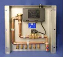
The Electronic Priming Assembly pictured is available in a single configuration but is capable of priming from thirteen to twenty separate floor drain traps from a single twenty one to thirty separate floor drain traps from a single control unit. The manifold is available in either 1/2" or control unit. The manifold is available in either 1/2" or 5/8" 5/8" compression fittings. This model serves 13 to 20 compression fittings. This model serves 21 to 30 drains. drains.
