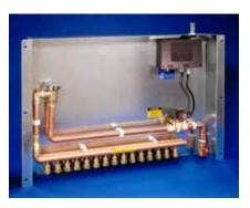
The PRIME-TIME PRIMING ASSEMBLY will supply a minimum of 2 oz. of potable water at 20 P.S.I.G. at a preset factory setting of 6 seconds every 24 hours. The entire unit is pre-assembled in a steel cabinet ready to be flush wall mounted.
