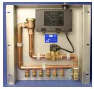
The Electronic Priming Assembly pictured is available in a single configuration but is capable of priming from twenty one to thirty separate floor drain traps from a single control unit. The manifold is available in either 1/2" or 5/8" compression and 1/2" PEX fittings. This model serves 21 to 30 drains.
