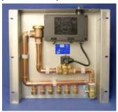
The Electronic Priming Assembly pictured is available in a single configuration but is capable of priming from twenty one to thirty separate floor drain traps from a single control unit. The manifold is available in either 1/2" or 5/8" compression, 1/2" PEX or PROPEX fittings. This model serves 21 to 30
