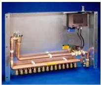
The PRIME-TIME PRIMING ASSEMBLY will supply a minimum of 2 oz. of potable water at 20 PSIG at a preset factory setting of 6 seconds every 24 hours. The entire unit is pre-assembled in a steel cabinet ready to be flush wall mounted.
